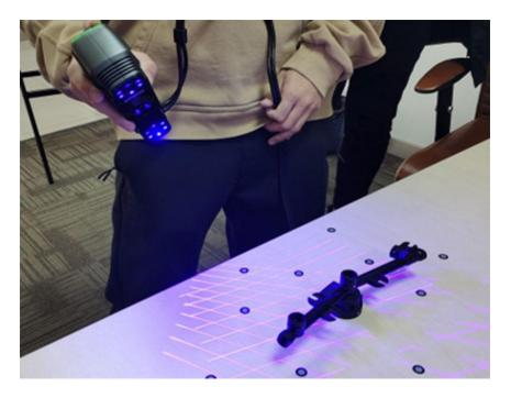
Complete and accurate data were obtained <u>when scanning black surfaces</u>, as shown below:
