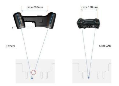
In this way, when scanning narrow spaces, both of the two cameras of the 3D scanner can see the laser lines projected on the object. The shorter camera distance helps SIMSCAN to perform better when scanning the narrow areas like the grooves. See the picture below to find out how it performs.
