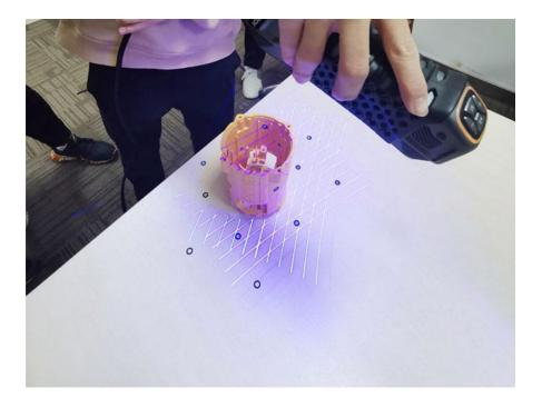
With an accuracy of up to 0.020 mm, SIMSCAN ensured the 3D data of these complex parts are precisely captured for further analysis.
