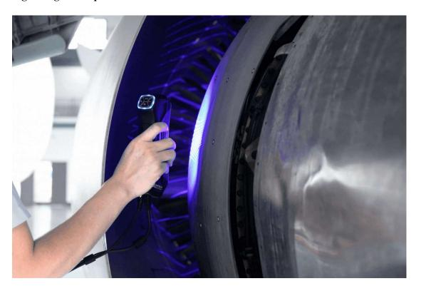
Portable 3D scanner SIMSCAN stands out among traditional measurement methods as it can be used both in lab and on shop floor. It is lightweight (750g) and portable, which can be carried around to cater to different needs, especially scanning in narrow spaces.
