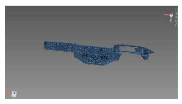
It is tedious and time-consuming to measure parts with traditional measuring methods like vernier, ruler, and micrometer. A few attributes, such as width, height, and depth, can be measured, while the surfaces' curvature and concave surfaces are challenging to measure. With handheld SIMSCNA, users can capture full-filed 3D data to get more insights of the product quality.
