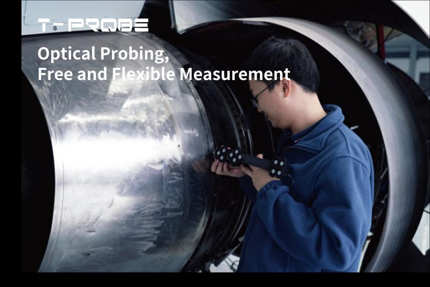
T-Probe is a portable CMM probing system that comes with the i-Tracker to obtain dimensions of features, such as reference holes and hidden points. It can be widely used in the measurement of fixtures, stamping parts, and marking for actual machining allowance.
